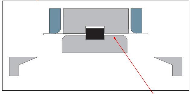
Firmly clamp and give ample support to the leads of the device in the forming jig while isolating the device body.
