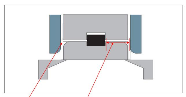
The distance between center of bending point and body must be more than 3mm and force less than 1KGF. Maintain firm pressure on leads next to body until bend is complete to avoid any excess mechanical stress to interior cavity.
